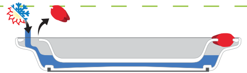
CROSS SECTION: FILL THE BASE WITH HOT OR COLD
