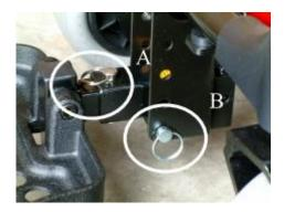
footrest slide tube and position the footrest at the required height. Three heights are available. Refit the connecting pin in the appropriate hole and make sure the connecting pin protrudes through the other side of the tube and is secure.
