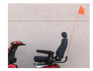
All of the above accessories come complete with all the necessary fitting required to fit the accessory securely to the under seat mounting point. The under seat mounting point needs to be 25mm x 25mm to accommodate these accessories.
